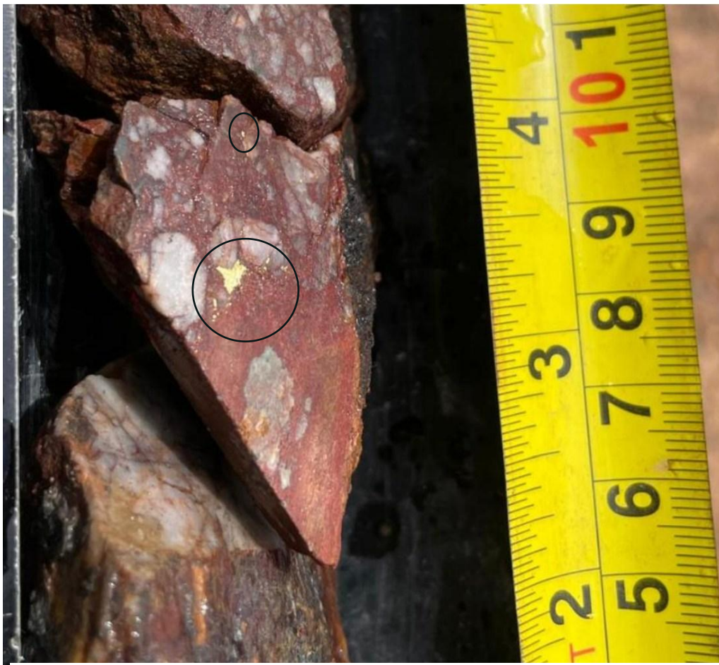
Plate 3: Close up of visible gold in oxidised brecciated quartz vein, intersected at 89.47m down hole in SDH25-009
