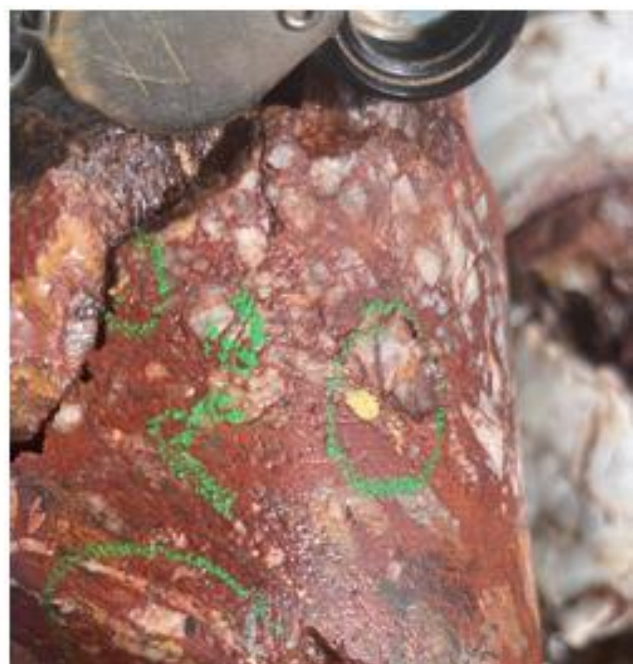
Plate 2: Visible Gold in oxidised brecciated quartz vein, intersected at 89.47m down hole in SDH25-009
