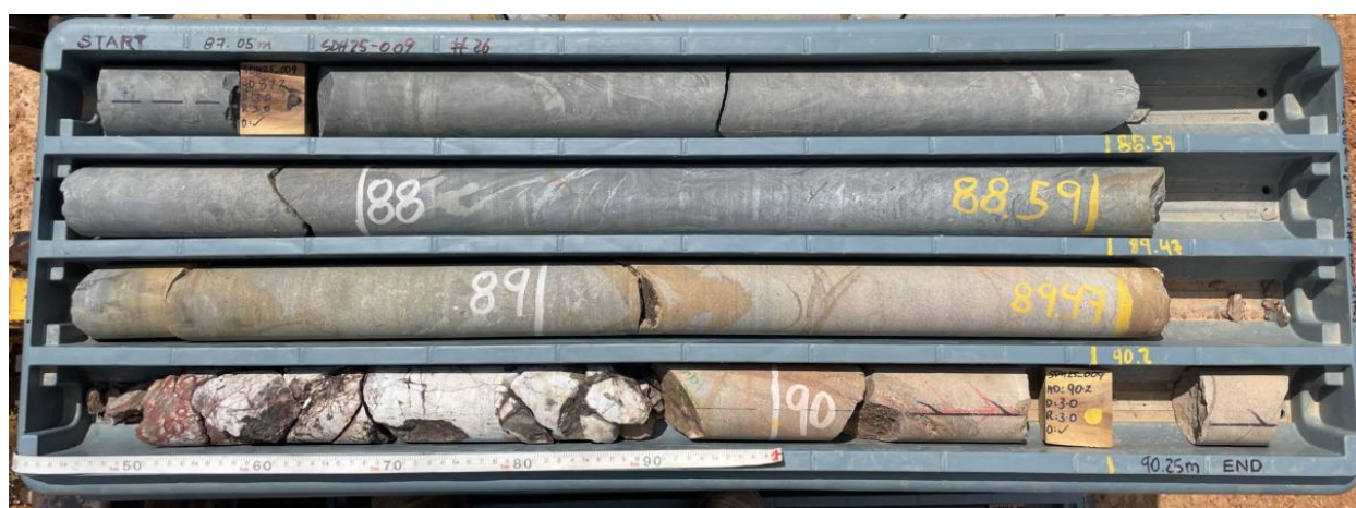
Plate 4: Drill core from SDH25_009, Au mineralisation 89.47m to 89.94m down hole
