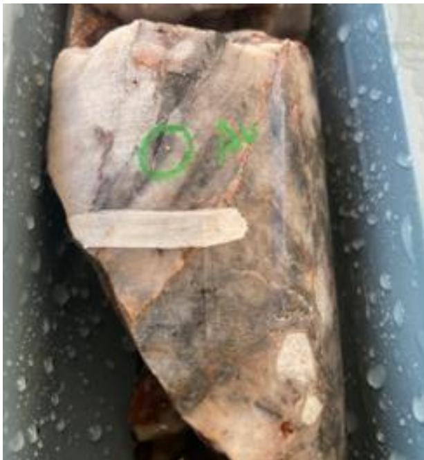
Plate 1: Visible Gold in laminated Quartz Vein, 122.5 m downhole in SDH25_006 breccia
